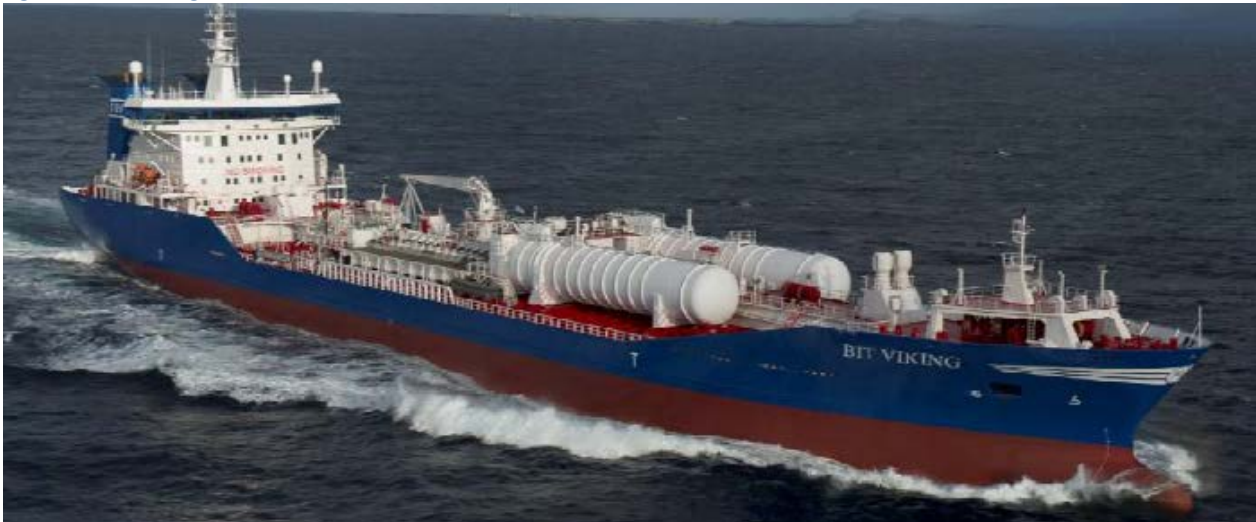
Figure 25. Bit Viking after conversion - LNG tanks on deck
