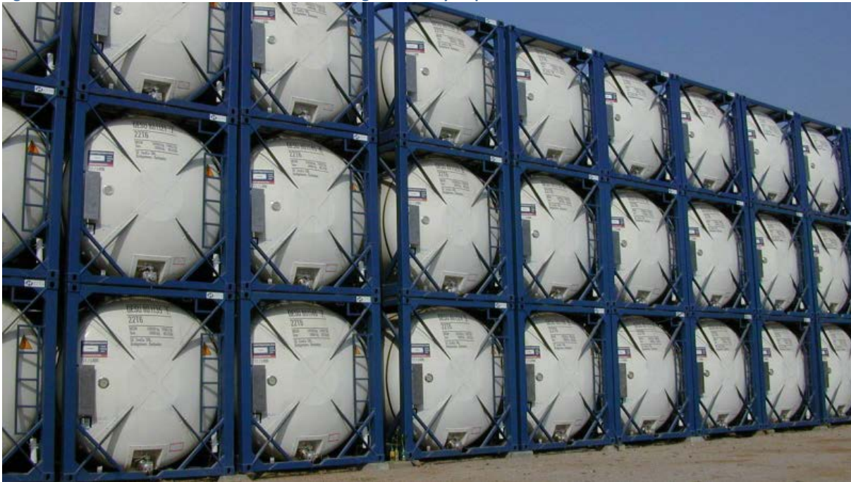
Figure 40. LNG containers for distribution and storage of LNG by ship and truck
