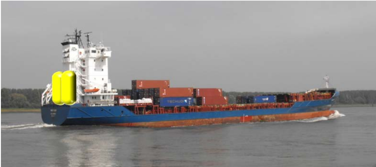
Figure 21 Fitting LNG tanks to an existing container vessel
