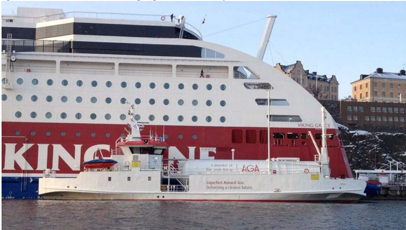
Figure 42. The first dedicated LNG bunkering barge in the world used by AGA in Stockholm
