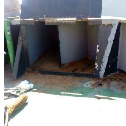
Heavy corrosion on STBD-FWD Bollard Pedestal
