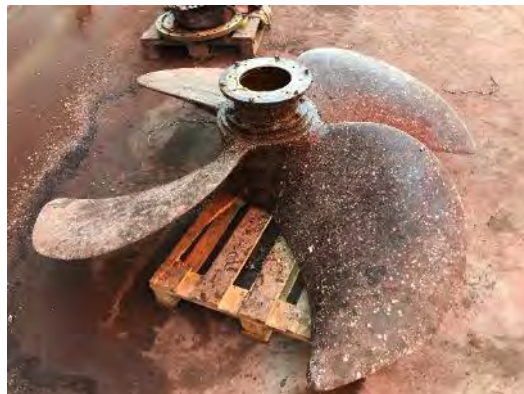
Steering and propulsion Propeller polishing post inspection
