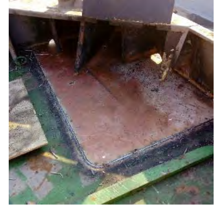
Steel replacement on STBD-FWD Bollard Pedestal
